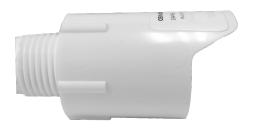
The Lux Meter/Photo Sensor provides the necessary daylight-level information to the Fixture Module. Using a photodiode element, this sensor continuously measures daylight levels and sends the information to the fixture module.
