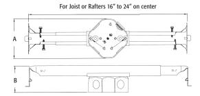
Mounts easily and securely between joists...adjusts from 16" to 24" o.c.
