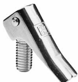
Provides quick access to Type 4 and 4X floor-mount and free-stand enclosures with clamps. The 3/8-16 threaded, stainless steel toggle latches replace the standard stainless steel bolts. Operation of the toggle releases the door clamp so the door can be opened without tools. Two Type 316 stainless steel toggle assemblies included.
