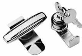
To install, simply remove the standard slotted latch and insert the kit. Complete installation instructions are furnished. Catalog number AL7A includes a Type L7 T handle and all hardware. Catalog number AL12AR includes a Type L12 cylinder lock, cam and all hardware. Latch and lock fit Type 1 enclosures and hinged-cover pull boxes.
