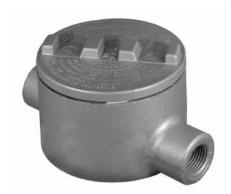
◆ In Class I, Division 1, Group B atmospheres, all conduit runs must have a sealing fitting (not supplied) field-installed adjacent to the enclosure.
