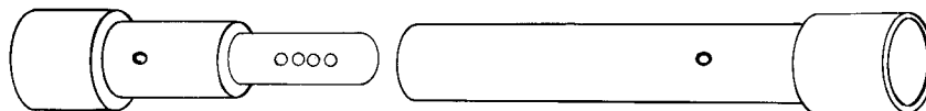
400 Amp 1.25" Solder Wire Well Terminals. Solid Copper Contacts with Four Spring-Loaded Borosilicate Bearings.
