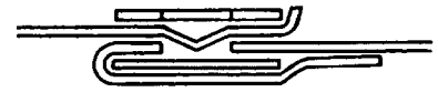
The tail is formed into a fold lock behind the buckle. The tool forces a dimple in the band into a hole in the buckle.
