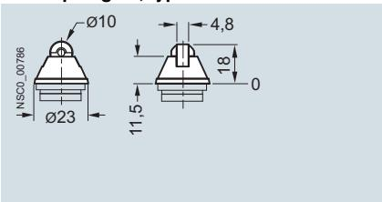
**Roller plunger with central fixing**
