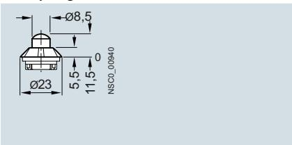
**Rounded plungers, type B acc. to EN 50041**
