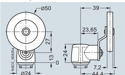
**Twist lever, rubber roller 50 mm**
