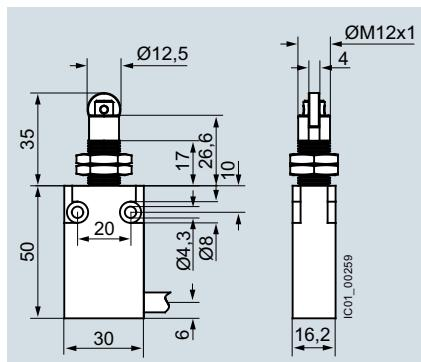
Twist lever, enclosure width 30 mm,
