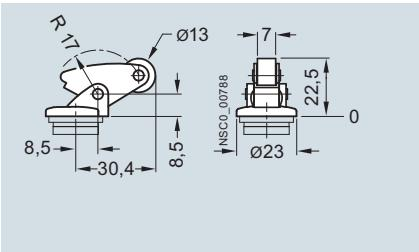
**Twist levers, type A acc. to EN 50047**
