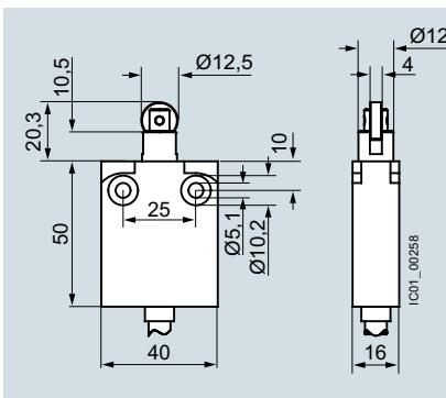
Roller plunger, enclosure width 30 mm,
