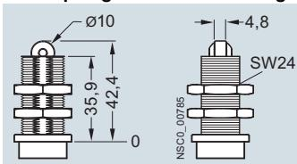
**Roller levers, type E acc. to EN 50047**
