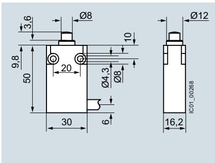
Rounded plunger, enclosure width 40 mm,
