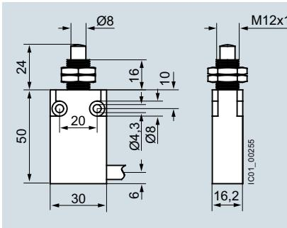
Rounded plunger, enclosure width 30 mm,
