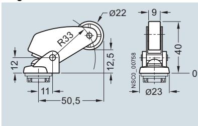
**Twist levers, type A acc. to EN 50041**
