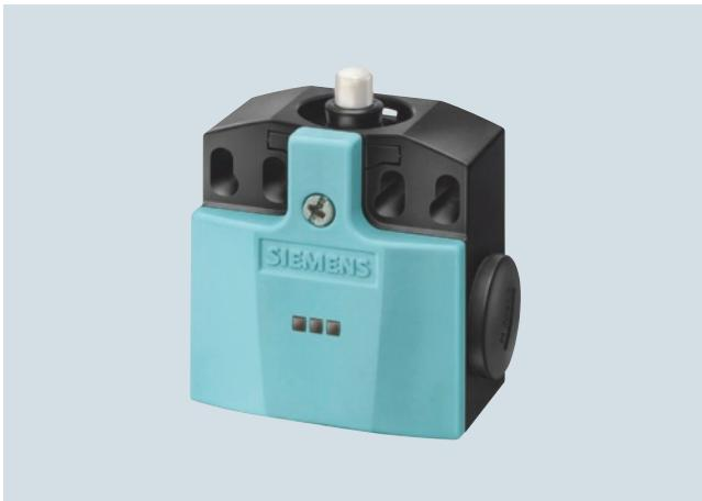
The enclosures are supplied with an LED signaling indicator (1 x green + 1 x yellow). This is the first time that optical signaling equipment is also available for small standard enclosures according to EN 50047. The LED signaling indicators are implemented in 24 V DC and 230 V AC.
