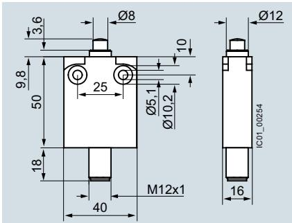
Rounded plunger, enclosure width 30 mm,
