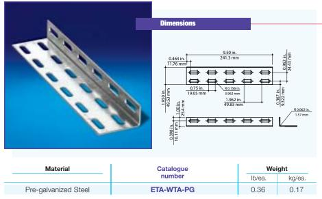
Support and terminate runs of cable tray with this wall termination angle. Can be used as a wall support, floor to ceiling support or to safely terminate any tray run. Adapts to any configuration and any width. Available in pre-galvanized steel. Mounting hardware sold separately.
