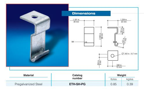
The side hanger clamp is used to construct trapeze supports using threaded rods. The offset support hole allows for trouble-free access to support nuts for height adjustment and the rod can continue downward to allow for multi-level (tiered) trapeze installations. A set screw holds tray firmly in position once installation is complete. Available in pregalvanized steel. For use with ¼" threaded rod.
