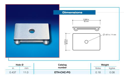
This clamp is used for center-hung applications to secure tray sections to threaded rod for ceiling mounting and can be used with U-profile tray in 4", 8" and 12" widths. This clamp is not designed for use with C-profile tray. Available in pregalvanized steel. For use with %" threaded rod.
