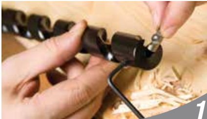
1 Insert Cutting Edge...
