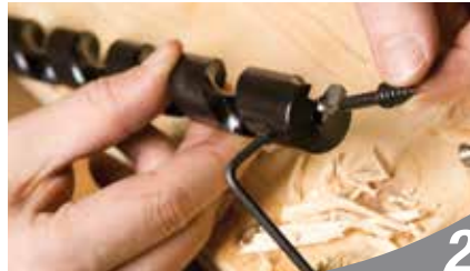
2 Insert Feed Screw...
