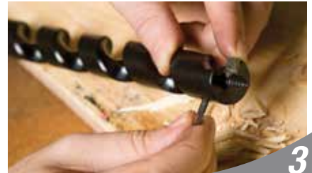
3 Tighten Set Screw.
