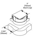
For right angle turns around external corners. Maintains 1 1/4" [32mm] bend radius when installing UTP and fiber optic cable. Also available in white (2918FO-WH).
