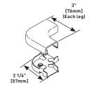
Makes right angle turns in 2800 Series Raceway on same surface. Maintains 1 1/4" [32mm] bend radius when installing UTP and fiber optic cable. Also available in white (2811F0-WH).
