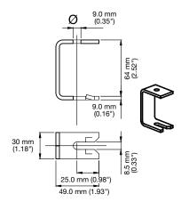
FESBS: 316 stainless steel - Set of two brackets for surface mounting
