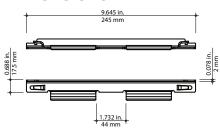
Connect straight lengths up to 24 in. wide using only two quick splices – no other components required. Simply bend tabs down and lock into position using pliers. Compatible with all profiles, the Quick Splice is available in pre-galvanized steel, hot-dipped galvanized steel and stainless steel (Type 316).
