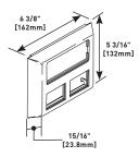
For mounting deeper devices such as TVSS receptacles, GFCI devices, and Pass & Seymour® Activate inserts. Accepts 5507 Series™ Faceplates, Ortronics® TracJack, and Series II Inserts. Bezels included. Available in white (5007C-2RTWH), black (5007C-2RTBK), or gray (5007C-2RTGY) PVC finishes.
