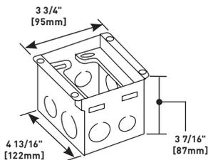
Knockouts for three (3) 1/2" [12.7mm], five (5) 3/4" [19.1mm], and two (2) 1" [25mm] conduits. 53 cu. in. [869ml] of capacity.
