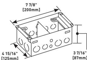
Knockouts for six (6) 1/2" [12.7mm], eight (8) 3/4" [19.1mm], and two (2) 1" [25mm] conduits. 58 cu. in. [951ml] of capacity in one compartment. 59 cu. in. [967ml] of capacity in second compartment. Barrier is removable for greater capacity if needed.
