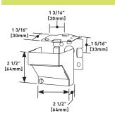
For feeding raceway from ceiling or floor. Allows for ample splice room. Base has 1/2" trade size KO.
