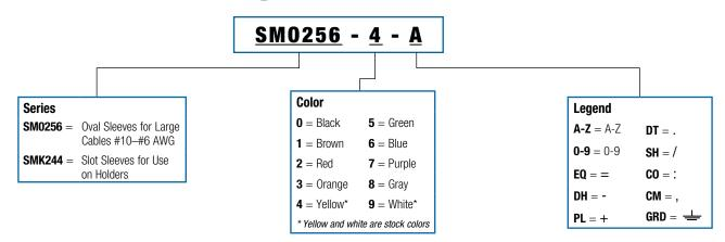
Example: The catalog number shown above is for yellow oval sleeve markers imprinted with the letter A for use directly on #10-#6 AWG cables or on SMOH or SMKH holders.
