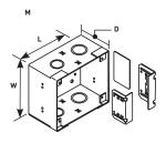
Slide-in dividers separate the box for power and communication services. Adjustable mounting brackets offer flexibility to flush mount box in 1/2", 5/8", 1", and 1/4" [12.7mm, 15.9mm, 25mm, and 32mm] wall thicknesses.
