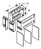
Slide-in dividers separate the box for power and communication services. Adjustable mounting brackets offer flexibility to flush mount box in 1/2", 5/8", 1", and 1 1/4" [12.7mm, 15.9mm, 25mm, and 32mm] wall thicknesses.
