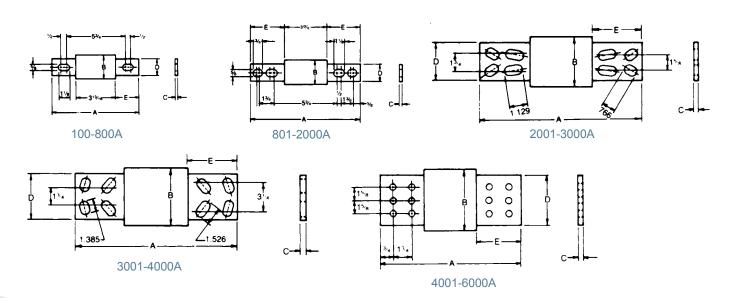
Safety Note: Class L fuses are dimensioned for one-way interchangeability. A Class L fuse of any lower ampere rating can be substituted for a given Class L fuse.
