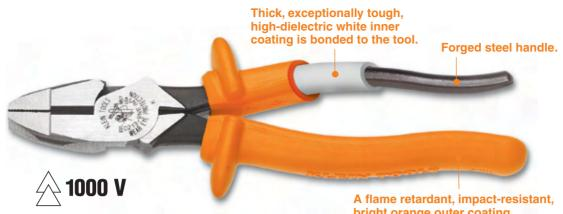
The line of insulated tools incorporates all the Klein quality design and construction features that professionals have relied on. The tools combine excellent functionality along with reduction of risk of injury where a tool might make contact with an energized source with voltage up to 1000 volts.
