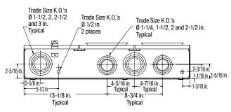
Note: Pattern for bottoms. Left hand entry is shown. For right-hand entry, unit is manufactured symmetrically with hub openings, knockouts for line connectors on right side.
