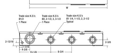
Note: Pattern for bottoms. Left hand entry is shown. For right-hand entry, unit is manufactured symetrically with hub openings, knockouts for line connectors on right side.
