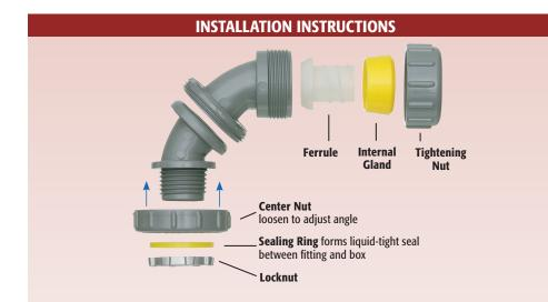
Arlington's no-spin ferrule allows the Zero to 90 connector to be secured to the conduit while fully assembled. To install, simply loosen the tightening nut and screw onto conduit. A positive liquid-tight seal is formed by the pressure sensitive internal gland as the nut is tightened. The sealing ring assures a liquid-tight seal between the fitting and box.
