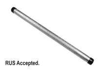
Single-sleeve aluminum UNISPLICE™ designed to splice ACSR as simply as all aluminum. Pre-filled with PENETROX™ joint compound, stripsealed and capped to limit oxide growth and to increase the life of the connection. Eliminates strand stripping, installing separate steel sleeve
