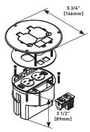
Includes round PVC floor box, one 15A, 125V tamper-resistant duplex receptacle, one coax F connector, one RJ45 Category 5e connector, and brushed aluminum duplex opening cover plate with two flip lids.
