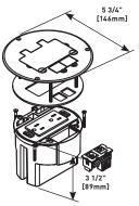
Includes round PVC floor box, one 15A, 125V tamper-resistant decorator style duplex receptacle, one coax F connector, one RJ45 Category 5e connector, and brushed aluminum duplex opening cover plate with single flip lid.
