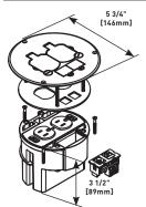
Includes round PVC floor box, one 15A, 125V tamper-resistant duplex receptacle, one coax F connector, one RJ45 Category 5e connector, and brass duplex opening cover plate with two flip lids.
