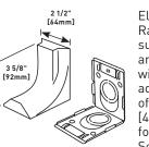
Eliminates offsetting 2400 Series Raceway in connecting with surface panel boxes. Has 3/4" and 1" concentric trade size KOs with 1" trade size KO elongated so adjustment from surface to center of bushing is 1" [25mm] to 1 5/8" [41mm] maximum. Has twistouts for transition to 1500 and 2600 Series Raceway.
