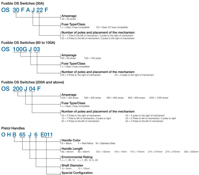
E011 = 3 position transfer switch handle EH = Stainless Steel Hasp
