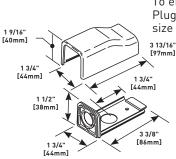
To end feed raceway or Plugmold strip. Has 1/2" trade size KO on end and bottom.
