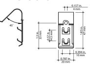
Secure covers to tray quickly with this cover clip. Available in stainless steel (type 316), the cover clip uses built-in tabs to secure the cover and to facilitate removal of the cover when required. No tools required.
