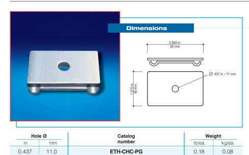
This clamp is used for center-hung applications to secure tray sections to threaded rod for ceiling mounting and can be used with U-profile tray in 4", 8" and 12" widths. This clamp is not designed for use with C-profile tray. Available in pregalvanized steel. For use with %" threaded rod.
