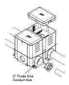
Box comes complete with reusable mudcap, insert spacer, conduit plugs and reducers. Reducers provided for reduction to 1 1/2", 1 1/4", 1", 3/4", and 1/2" [25mm, 19.1mm, and 12.7mm] conduit. Minimum concrete depth is 4" [102mm] and maximum concrete depth is 6" [152mm]. Minimum capacity is 50 cu. in. [819ml] and maximum capacity is 100 cu. in. [1693ml]. Box dimensions are 4 1/8" W x 5 1/2" L x 6" H [105mm W x 140mm L x 152mm H].
