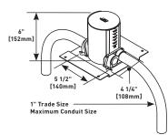
Supplied with reusable concrete cap, conduit reducers, and conduit hub plugs. Available for single service only. Graduated cubic inch markings inside the box indicate volume capacity at any depth. Box has parallel conduit hubs eliminating the need for 90° sweeps in installation. One-piece reduction from 1" to 1/2" [25mm to 12.7mm] conduit. Reducers and plugs located on a mounting bar for easier selection. For concrete pours of 2 1/4" to 6" [57mm to 152mm].
