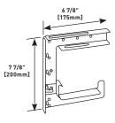
Suspends S4000, 4000 or 6000 Series Raceway from a structural ceiling. Designed for use with 3/8" [9.5mm] rod. Hangers should be installed no more than 5' [1.5m] apart along raceway run. Can be bolted back-to-back for dual runs of 3000, 4000 or 6000 Series Raceway.
