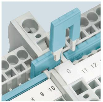
Reducing combs enable easy connection of terminals with various nominal cross-sections. For example, they can be used for the fast creation of infeed blocks, e.g. by connecting a 10 mm² spring-loaded terminal with a 2.5 or 4 mm² spring-loaded terminal.
