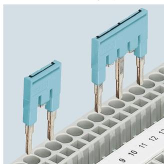
Contact tabs can be removed from the standard comb in order to skip individual terminals. This means that two potentials can run in parallel on a single terminal strip. The contact points can additionally be marked.
