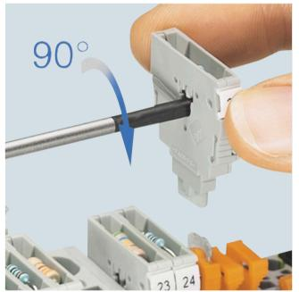
The component connector enables the convenient equipping with electronic components. One turn of the screwdriver opens the contact points and the component is easily inserted.
