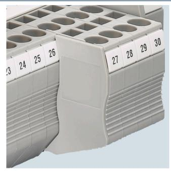
Cover segments are used to cover the projecting terminal segments of three and four-wire terminals when mounting two-wire terminals side-by-side. This ensures touch protection.
