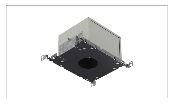
The 2-010 series housing is designed for insulated and airtight ceilings. Performing in accordance with ASTM E283-91, the airtight option also meets the requirements of "having no more than 2.0 CFM air movement from the conditioned space to the ceiling cavity" (Sec. 502.4 of 1991 WSEC—Washington State Electrical Code).
