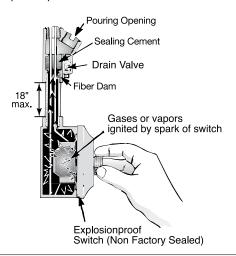
Appleton sealing fittings are suitable for Class I and II locations. EYS, SF and EYD are for sealing vertical conduit. EY and ESU are for sealing vertical and horizontal conduit. SF and EYD also have drain valves.
