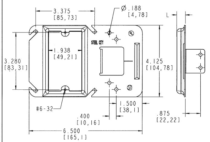
MATERIAL: PRE-GALVANIZED STEEL 0.063" THICK
