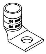
WIRE SIZE: 300 MCM, 4/0 WELD, 650/24 MATERIAL: HIGH CONDUCTIVITY COPPER
