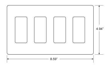
Align subplate over NEMA 26 sized electrical devices and receptacles. Affix subplate with included screws to electrical wall box. Secure tightly, but avoid over torquing screws. Snap on radiant screwless wall plate to subplate.
