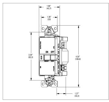
Figure 9. SGFD20 Line art with dimensions
