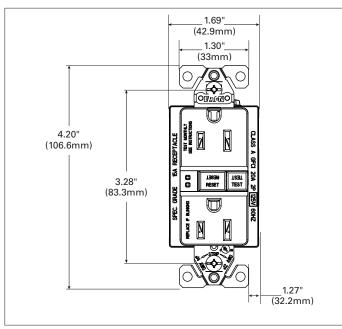
Figure 1. SGF15, SGF15-M & SGF15F Line art with dimensions
