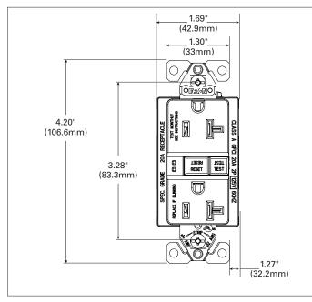
Figure 5. SGF20 & SGF20F Line art with dimensions
