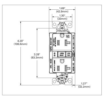
Figure 8. TWRSGF20 Line art with dimensions
