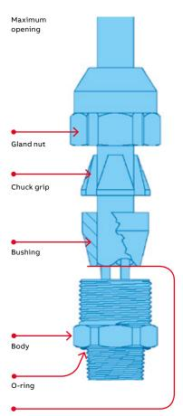
\*When cord will not fit through body, strip cord jacket and trim fillers if required. Insert cable ensuring the outer jacket reaches the end of the bushing as shown. Tighten gland nut onto body
