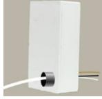
STEP 2 Punch out desired 1/2" knockout(s) - Part #1 from the back of the box. Insert your preferred choice of approved type cable connector(s). Bring wiring/cable(s) into the box.
