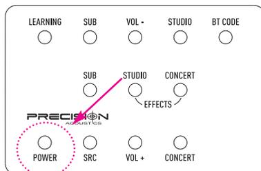
Press the POWER button on the sound bar and the LED in front of the sound bar will stop flashing. The POWER function of the sound bar can now be controlled by pressing the Number 1 key on your remote. / Appuyer POWER sur le bar de son et la lumière va arrêter à clignoter.
