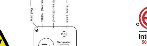
Suitable only for use with generators that do not have the neutral bonded to ground or the generator frame Warning: More than one live circuit For use by "Qualified Personnel Only"
