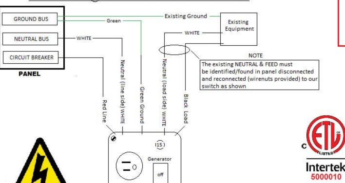
Suitable only for use with generators having the neutral bonded to ground or the generator frame Warning: More than one live circuit For use by "Qualified Personnel Only"
