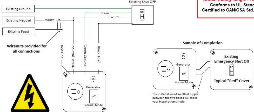
Suitable only for use with generators that do not have the neutral bonded to ground or the generator frame Warning: More than one live circuit
