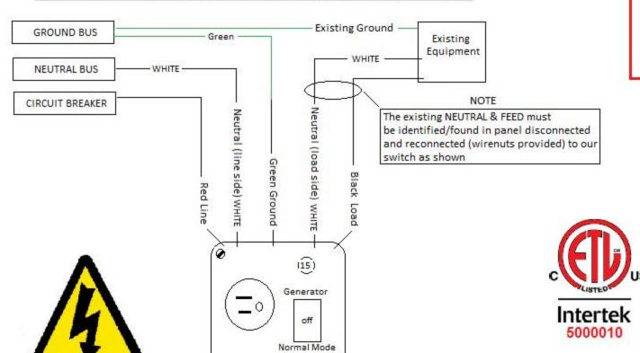
Suitable only for use with generators having the neutral bonded to ground or the generator frame Warning: More than one live circuit
