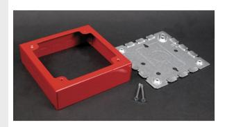
For surface mounting of alarm devices and safety signals designed to fit into 4" [102mm] square back boxes. Cover has three raceway twistouts on each side. Base has 1/2" and 1" concentric and single-gang box KOs. R5752 has red finish. Accepts NEMA double-gang standard faceplates.
