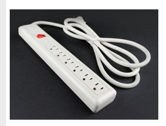
Six outlets, putty white impact-resistant polymeric housing, 15A, lighted switch. 6' [1.8m] 14/3 SJT putty white cord with NEMA5-15 plug. Length 12" [305mm]. Receptacle center-to-center 1 1/4" [32mm]. Keyhole mounting.
