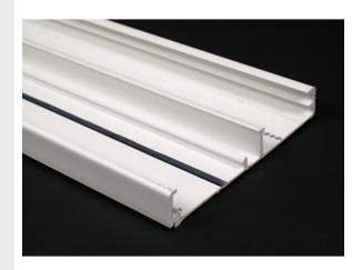
5000B Base has an integral divider forming two channels for power and low-voltage separation. Base supplied in 8' [2.44m] lengths, packed 80' [24.4m] per carton. (Base is not visible in a typical finished installation.)
