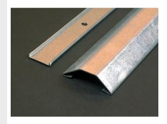
Cover: .050" galvanized steel. Base: .040" [1.0mm] galvanized steel. Packed five 10' [3m] lengths per carton. Base has 9/32" [7.1mm] diameter mounting holes on centers of approximately 8" [203mm].
